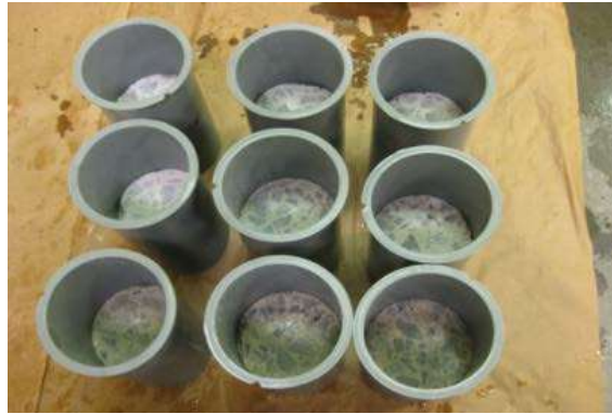
Fig. 2: Cylindrical specimen of substrate concrete inside the forms
