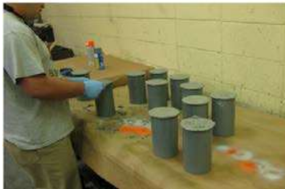
Fig. 3: Cylindrical specimen for overlay concrete
